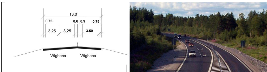
Figure 1: Typical 2+1 median barrier design on 12-13 m road
