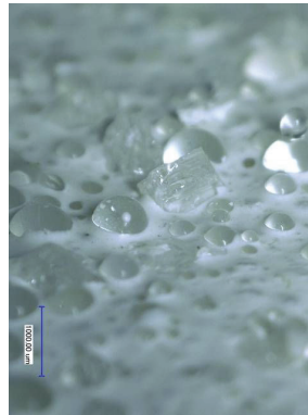
Fig. 1. Glass beads and antiskid aggregates embedded in a base road marking material.
