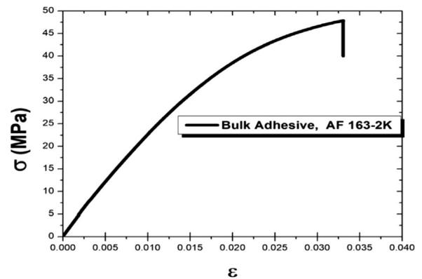
Fig. 3. Engineering tensile stress-strain curve for the adhesive film (AF163-2K).
