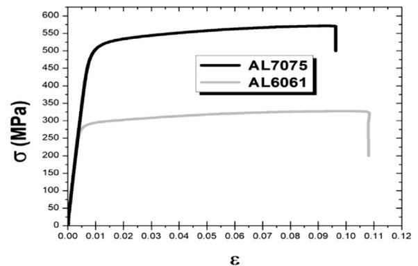
Fig. 2. Engineering stress-strain curves for the AL6061 and AL7075 adherends.
