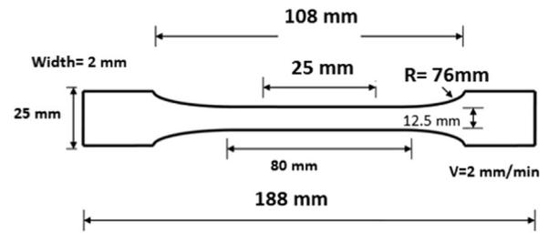
Fig. 1. Geometrical details of tensile test specimens for the aluminium adherends and the adhesive material.
