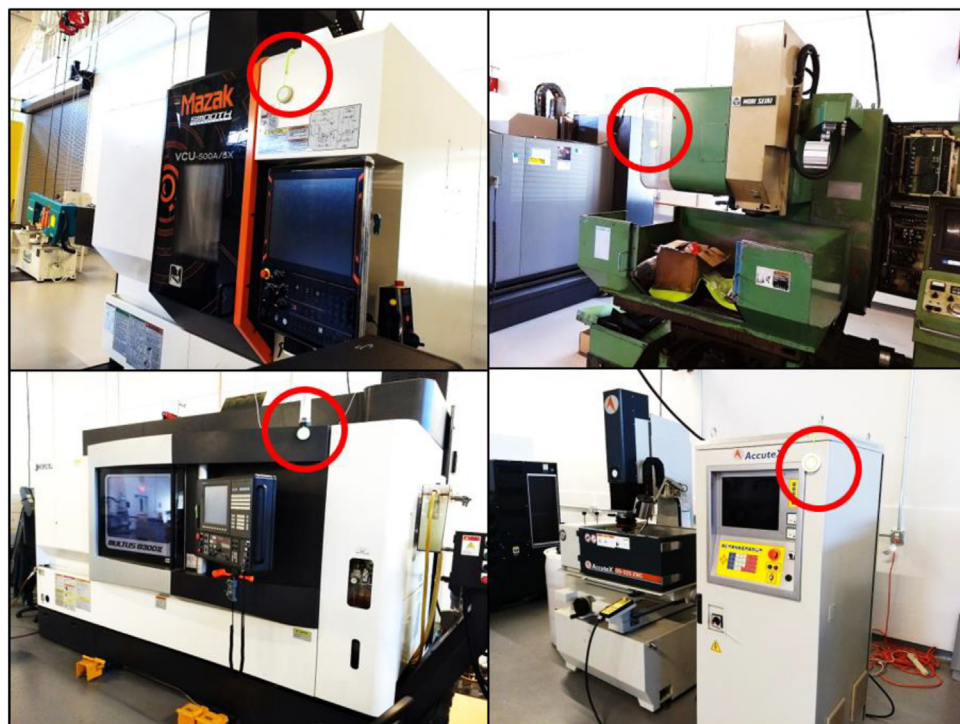
Fig. 2. Cutting machines with the BLE beacons (red circles) on them (For interpretation of the references to colour in this figure legend, the reader is referred to the web version of this article).
