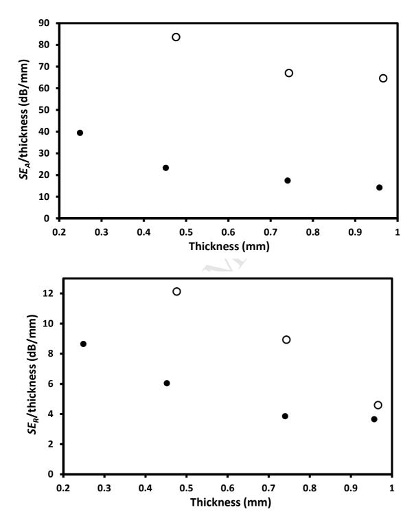
Effect of fiber lay-up configuration on the absorption loss ( $SE_A$ ) and reflection loss ( $SE_R$ ) at 1.0 GHz. Solid circles: unidirectional composite. Open circles: crossply composite.
