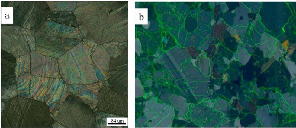
**Fig. 1.** Microscopic images showing grain structures in rocks. (a) A microscopic scanning image of a thin section of marble from Henan, China [36]. (b) Polarized and fluorescent image of LdB granite from the URL [18,37].
