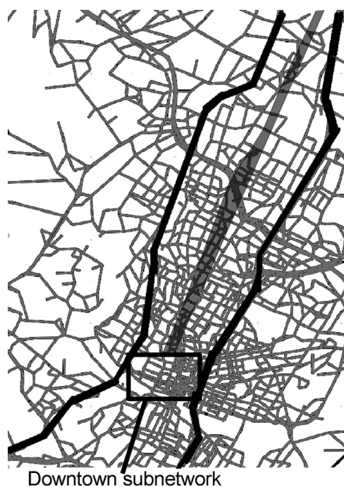
Fig. 1. Portion of regional network with equidistant region shaded. Route choice from this region to downtown is sensitive to changes in the subnetwork regardless of distance between the origin and downtown.
