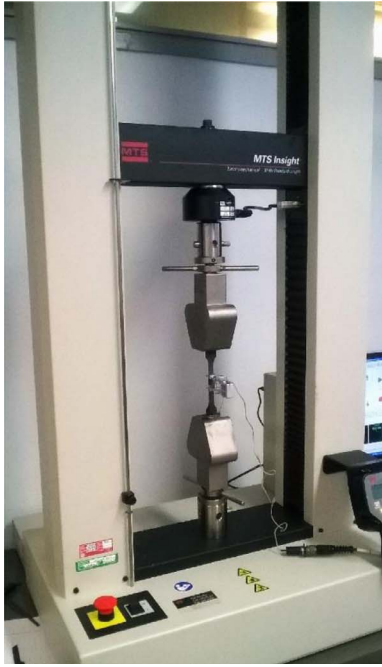
Fig. 1. Tensile testing equipment and test results in the rolling direction (RD) and orthogonal to rolling direction (ORD).
