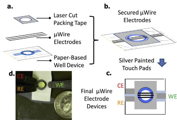
**Scheme 1.** Well-based ePAD fabrication showing (a) the device layers, (b) resulting side view of the device, (c) top view of the fabricated device with alternately covered and silver painted electrode ends, and (d) device image with electrode leads attached and 30  $\mu\text{L}$  of solution in the 7 mm diameter well.
