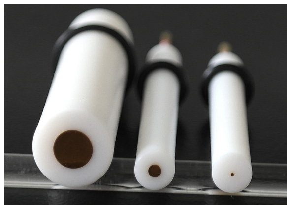
Fig. 1. The picture of 3 Au electrodes with different size ( \Phi = 6, 2, 0.5 mm).
