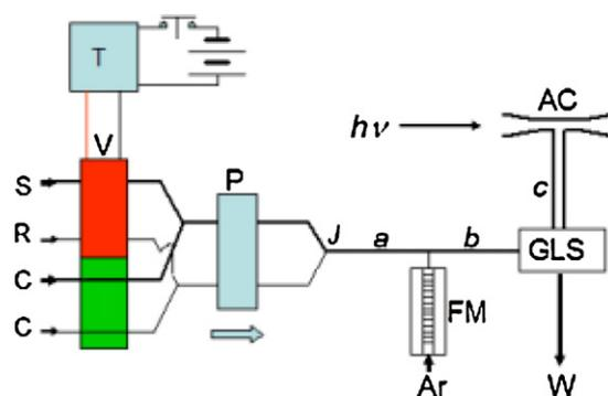
**Fig. 1.** FI-CCV-AAS system used for Hg determination. T: time delay relay; V: pinch valve; P: peristaltic pump; GLS: gas-liquid separator; AC: absorption cell; FM: flow meter; J: joining point; a and b: tubular reactors; c: gas delivery tube; S: sample; R: reductant (NaBH<sub>4</sub> solution); Ar: argon gas; C: carrier stream; W: waste.
