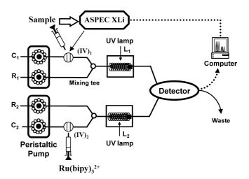
Fig. 1. Schematic diagram of the FI manifold.  $C_1$  and  $C_2$  = water;  $R_1 = 0.05 \, \text{mol} \, L^{-1}$  phosphate buffer of pH 6.5;  $R_2 = 1.5 \times 10^{-3} \, \text{mol} \, L^{-1}$  potassium peroxydisulfate and  $0.05 \, \text{mol} \, L^{-1}$  phosphate buffer of pH 5.7; (IV)<sub>1</sub> and (IV)<sub>2</sub> = injection valves;  $L_1$  and  $L_2$  = photoreactors.
