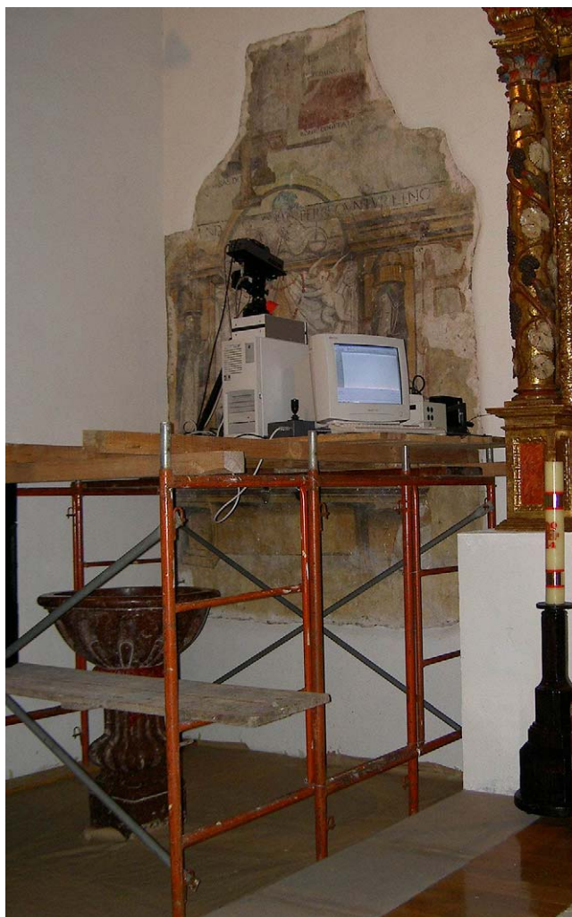
Fig. 1. Experimental set-up with the Raman instrument on the scaffolding.
