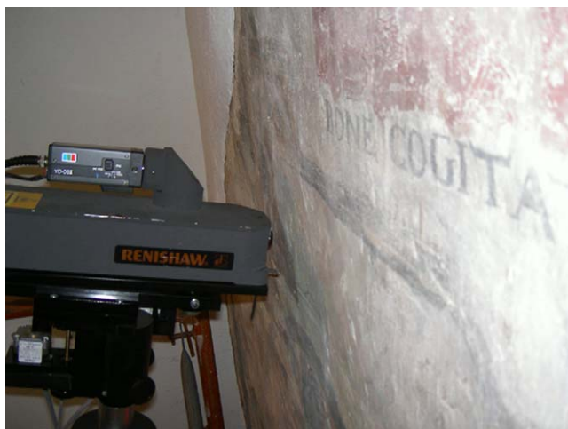
Fig. 2. Detail of the Raman probe at the working distance on the wall painting.
