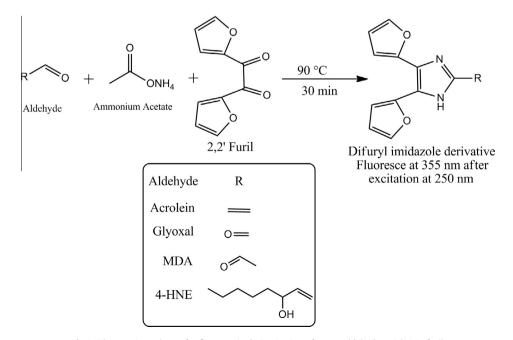
Fig.1. The reaction scheme for fluorogenic derivatization of target aldehydes with 2,2'-furil.
