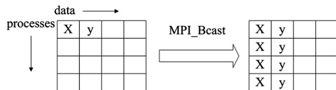
Fig. 1. Broadcast the training set of spectra and the standard concentration matrix to cores using the MPI_Bcast subroutine, each row represents data locations in a different process. At the beginning, the training set of spectra \mathbf{X} and the standard concentration vector \mathbf{y} are located only in process 0, after the calling of MPI_Bcast, they are replicated in all processes.
