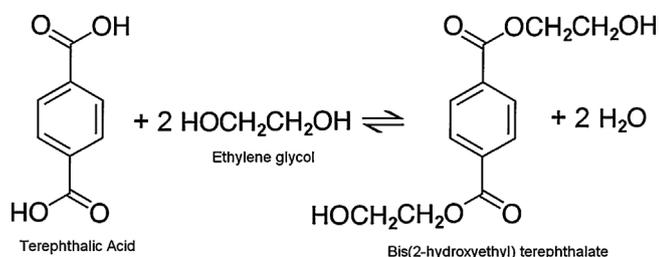
Fig. 1. Scheme of esterification of terephthalic acid with ethylene glycol.
