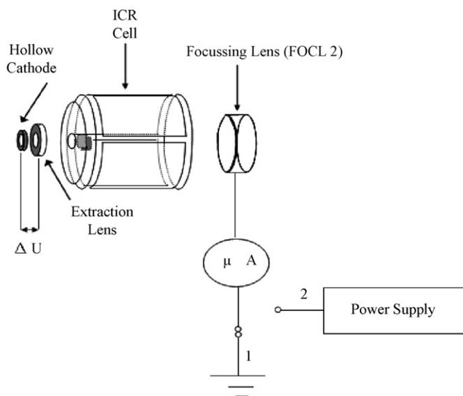
**Fig. 1.** Experimental configuration for electron current and energy measurements. The microammeter was connected to ground (1) when measuring electron current through the ICR cell, and connected to a floating power supply (2) when measuring the electron energy distribution.
