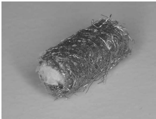
Fig. 1. The implant as used for this study. Titanium fibre mesh material was used to make a cylinder of 1 cm in length, 3 mm inner diameter, and 5 mm outer diameter. The central space of the cylinder was filled with 20 mg of dry COLLOSS ® material.
