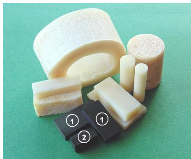
Fig. 1. Monolithic blocks cut from the bones: raw (light samples) and pyrolysed (black samples). Notation: ① –BB400, ② –PB550.
