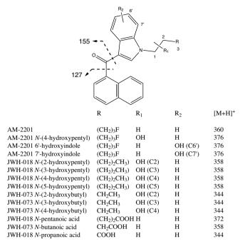
**Fig. 1.** Structures and *m*/*z* values of protonated molecules of AM-2201 and metabolites included in the method. The position of the hydroxyl group is specified in brackets. Cleavage sites for tandem mass spectrometry analysis are indicated by an arrow.
