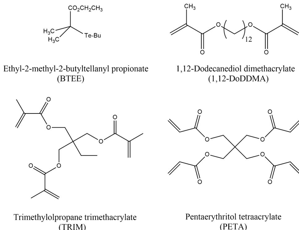
Fig. 1. Chemical structures of BTEE and multi-methacrylate/acrylate monomers.
