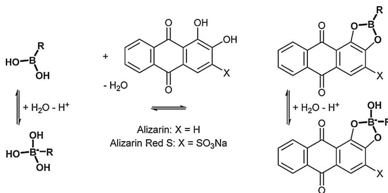
Fig. 1. Reaction of alizarin (or alizarin red S) with boronic acids to form a fluorescent complex.
