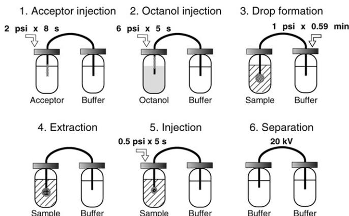
Fig. 1. Schematic of carried-mediated SDME.
