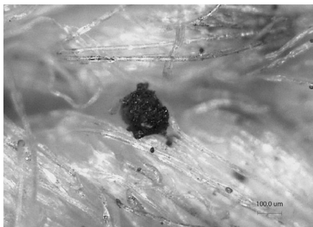
Fig. 1. Visual identification of partially burnt gunpowder particle was done at a high magnification (200 \times ) under a Keyence digital microscope.
