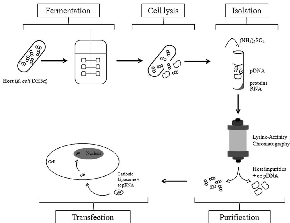
**Fig. 1.** Schematic representation of downstream processing of sc pDNA preparation, according to quantity and purity degree required for clinical applications, using lysine-affinity chromatography as a major purification step. *E. coli*, *Escherichia coli*;  $(\text{NH}_4)_2\text{SO}_4$ , ammonium sulfate; oc, open circular; sc pDNA, supercoiled plasmid DNA.
