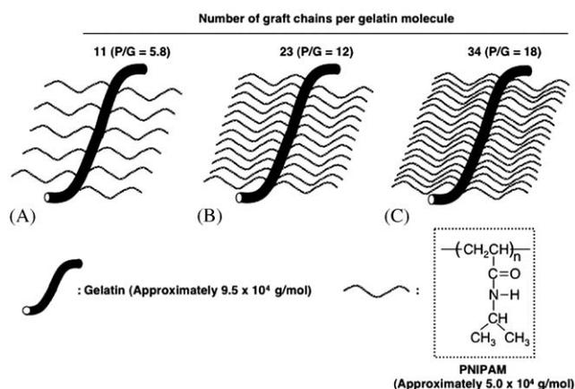
Fig. 1. Schematic structure of PNIPAM-gelatins with different graft chain densities.
