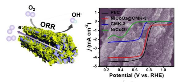
A novel NiCoO<sub>2</sub>@CMK-3 composite with nanosheets-shaped hierarchical structure was synthesized via a facile hydrothermal method. The as-prepared NiCoO<sub>2</sub>@CMK-3 composite exhibits comparable ORR electrocatalytic activity and better methanol-tolerance and electrochemical stability to the commercial Pt/C catalyst. The outstanding performance confirms the NiCoO<sub>2</sub>@CMK-3 composite as a promising efficient ORR catalyst in fuel cells and metal-air batteries.
