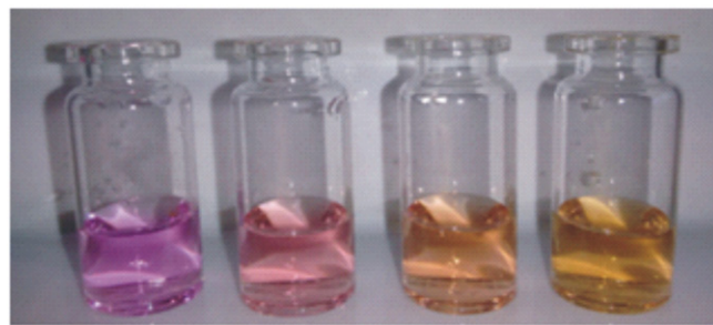
Fig. 2. Reaction of brightener in \text{HCl } 10^{-4} \text{ M} solution with \text{MnO}_4^- . 150 \mu\text{l} of a 3.2 mM \text{KMnO}_4 solution (pH = 4 with HCl) was added to 5 ml of the standards and left to react for 10 min. From left to right: 0, 0.3, 0.5 and 0.7 ml/l brightener, equivalent to 0, 0.34, 0.57 and 0.79 mM in o-chlorobenzaldehyde, respectively.
