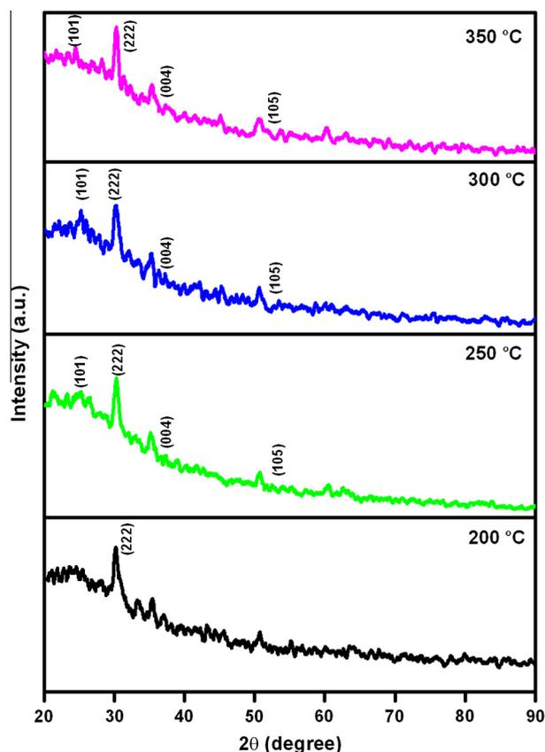
Fig. 1. XRD patterns of  $\text{TiO}_2$  films prepared on ITO coated glass substrate at different temperatures.
