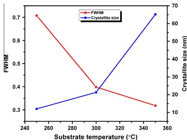
Fig. 2. Variation in crystallite size and FWHM of  $\text{TiO}_2$  films deposited on ITO coated glass substrate at different temperatures.
