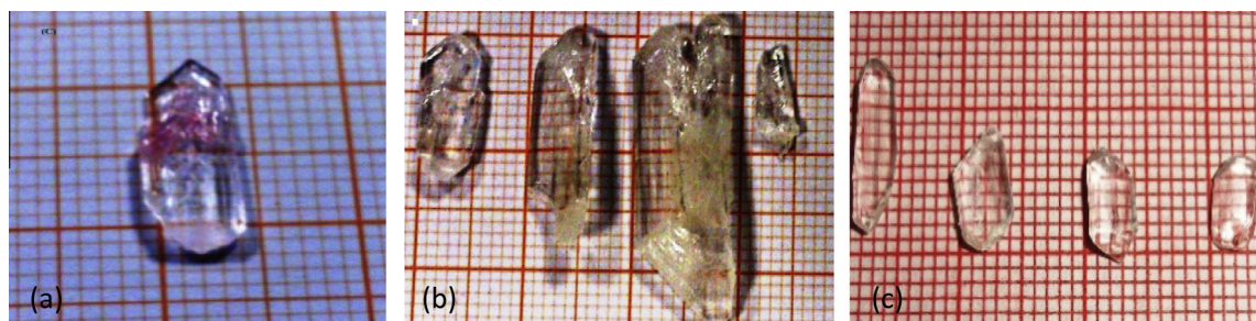
Fig. 1. Grown single crystals of (a) pure LPTCA (b) Ni 2+ doped LPTCA (c) Co 2+ doped LPTCA.
