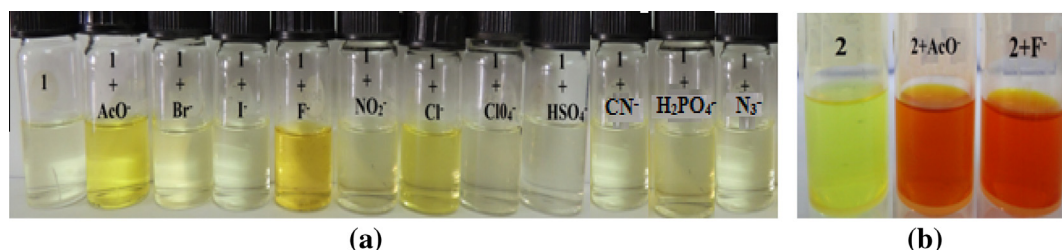
Fig. 1. Color changes observed: (a) receptor 1 on addition of various anions with a visible color change with fluoride and acetate only (b) receptor 2 on addition of fluoride and acetate respectively. (For interpretation of the references to color in this figure legend, the reader is referred to the web version of this article.)
