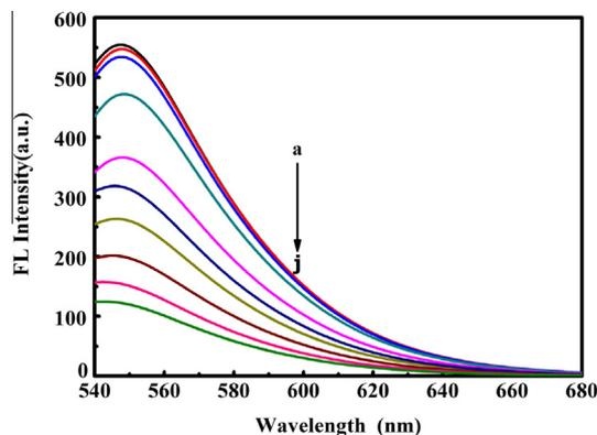
Fig. 1. Fluorescence emission spectra of eosin Y (curve a), eosin Y/PEI (curve j) and eosin Y/PEI/PFOS (curve b–i). Concentration: eosin Y ( $0.1 \times 10^{-6} \text{ mol/L}$ ), PEI ( $0.5 \times 10^{-6} \text{ mol/L}$ ), PFOS (i–b: 0.5, 0.8, 1.0, 1.2, 1.5, 2.0, 3.0,  $5.0 \times 10^{-6} \text{ mol/L}$ ). Britton–Robinson buffer solution, pH 7.0.
