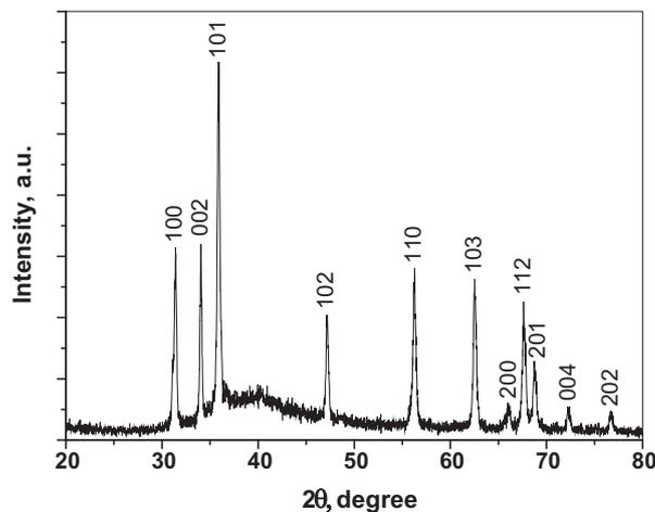
Fig. 1. XRD pattern of the ZnO sample synthesized by microwave-assisted hydrothermal technique.
