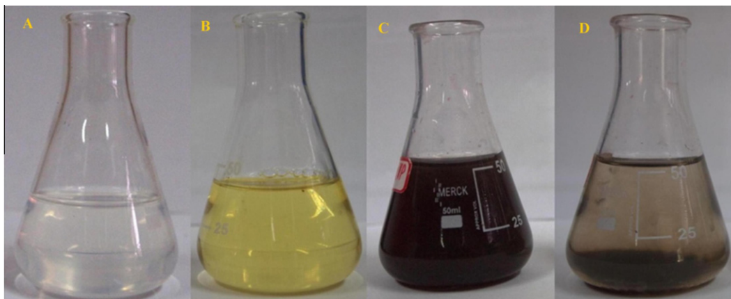
Fig. 1. Silver nitrate solution (A), plant extracts (B), synthesized silver nanoparticle after 5 min (C), silver nanoparticles settle down after 10 min.
