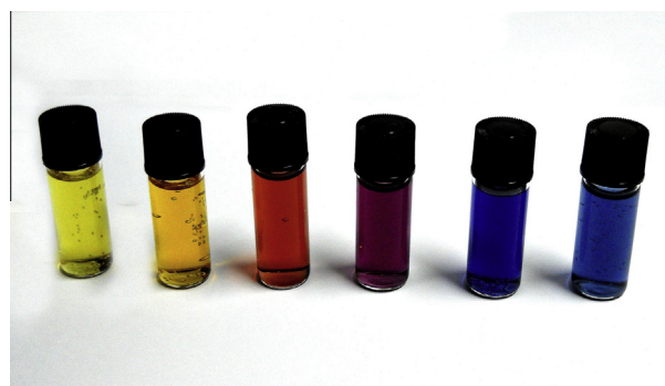
Fig. 2. Colloidal solutions from yellow to blue obtained by dilution of the KBr solution ( 2.75 \times 10^{-6} , 1.72 \times 10^{-6} , 1.38 \times 10^{-6} , 1.03 \times 10^{-6} , 6.90 \times 10^{-7} , 0.0 M). (For interpretation of the references to color in this figure legend, the reader is referred to the web version of this article.)
