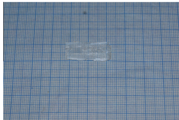
Fig. 2. As grown single crystal of EPAB.
