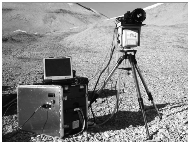
Fig. 2. A general overview of the Remote Raman prototype deployed at the field in the Svalbard Islands (Arctic) during AMASE 2008 and 2009 expeditions.
