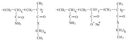
block [2,9]. The structure of block influences on the strength and stiffness of the gel [8].
