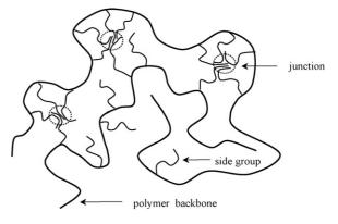
Fig. 1. Schematic image of the gel network junction created by hydrophobically modified polymers.
