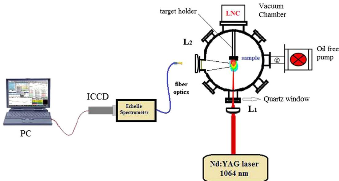
**Fig. 1.** Schematic diagram of the experimental setup [LNC, liquid nitrogen container, L<sub>1</sub> ( $f = 7.5$  cm); and L<sub>2</sub> ( $f = 5$  cm) are plano-convex collimating lenses].
