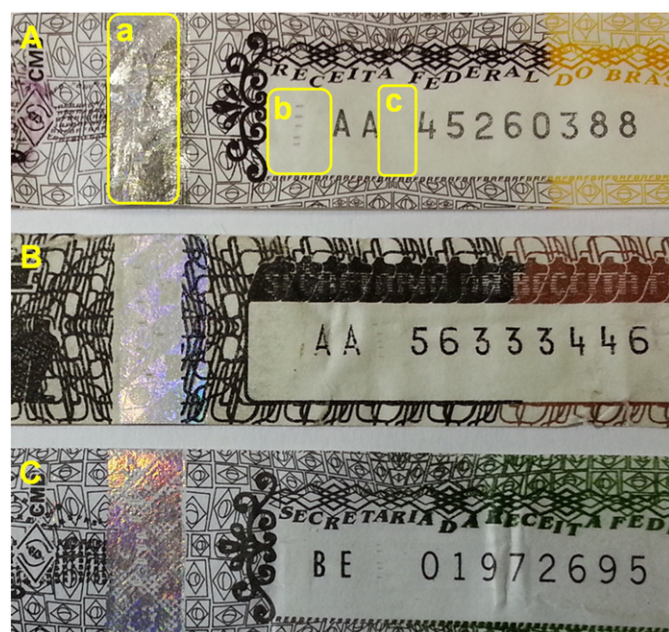
Fig. 2. Photographs of part of one authentic (A) and two false (B and C) tax stamp samples showing the sample regions used in the analysis: (a) hologram, (b) or (c) blank paper.
