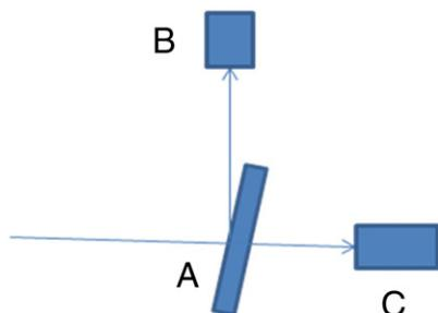
Fig. 1. Schematic lay-out of the experiment at the 2-ID-B beamline (APS, Argonne, USA). A: Sample; B: fluorescence detector; C: transmission detector.
