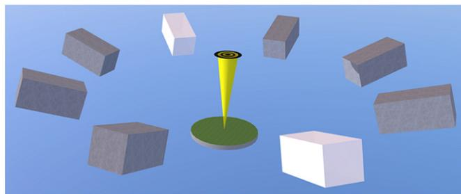
Fig. 2. Fluorescence detector geometry at the TwinMic beamline at Elettra (Trieste, Italy). The 8 Silicon Drift Detectors (SDD) are located in an annular configuration and their axis is tilted of 20° with respect to the sample plane. The 2 SDDs represented in white were not available during the measurements.
