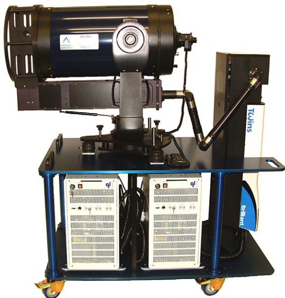
Fig. 1. Photograph of the double-pulse ST-LIBS system developed by ARL in collaboration with Applied Photonics, Ltd. and Ocean Optics, Inc.
