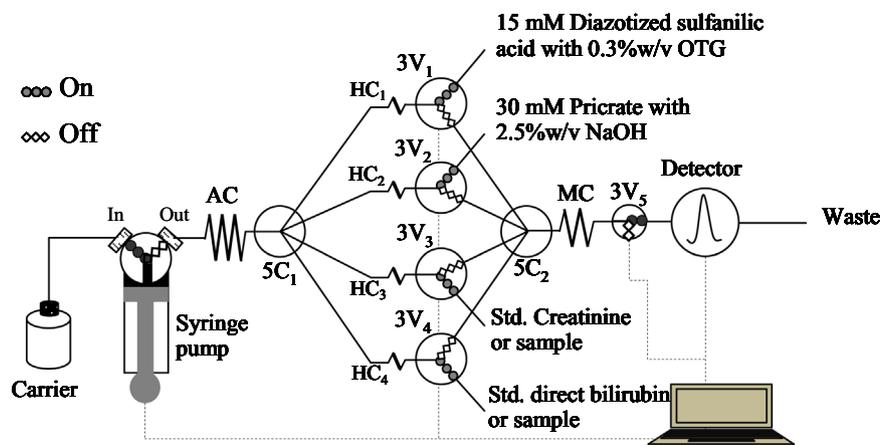
Fig. 1. The SIEMA system for successive urinary bilirubin and creatinine detection; AC, auxiliary coil (100 cm, 1.5 mm i.d.);  $5C_1$  and  $5C_2$ , 5-way cross connectors;  $HC_1$ ,  $HC_2$ ,  $HC_3$  and  $HC_4$ , holding coils (100 cm, 0.8 mm i.d.);  $3V_1$ ,  $3V_2$ ,  $3V_3$ ,  $3V_4$  and  $3V_5$ , 3-way solenoid valves; MC, mixing coil (100 cm, 0.8 mm i.d.).
