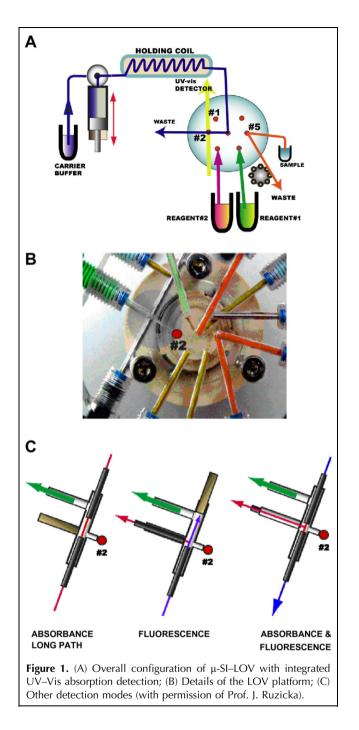
be integrated into the platform, depending on the detection technique. Integration of the multipurpose flow-cell, in which light measurements are carried out through optical fibers, means that the system is very versatile in measurements, although LOV can also be used with non-integrated cells for optical or electroanalytical measurements.
