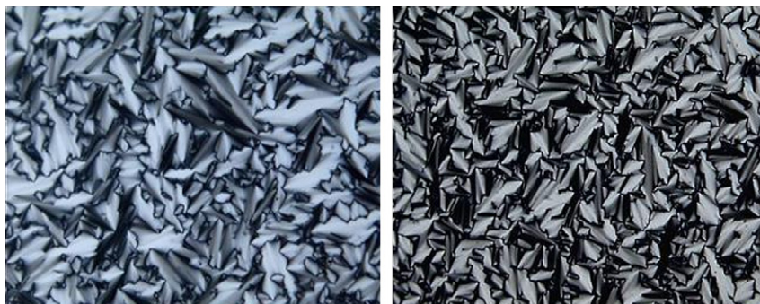
Fig. 1. The fan-shaped texture of the SmA phase obtained upon slow cooling of the isotropic liquid of C 13 -2d- \beta -Glc (left) and binary mixture C 12 -2d- \alpha , \beta -Glc (1:1) (right).
