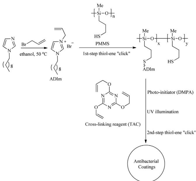
**Scheme 1.** Polysiloxane-based antibacterial polymer coatings prepared by a two-step sequential thiol-ene click chemistry protocol.
