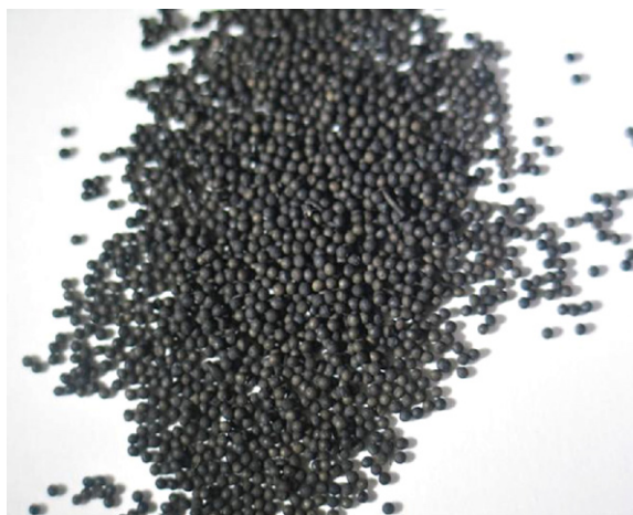
Fig. 1. Photo images of 1.0 wt% Pt/ \text{Li}_4\text{SiO}_4 pebble.
