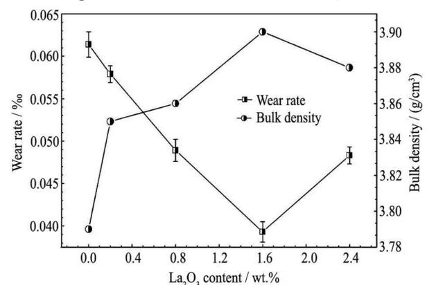
Fig. 2 Wear rate and bulk density curves of samples
