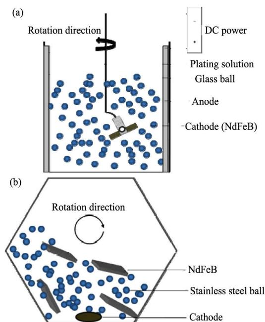
Fig. 1 Schematic diagrams of mechanical attrition electroplating devices
