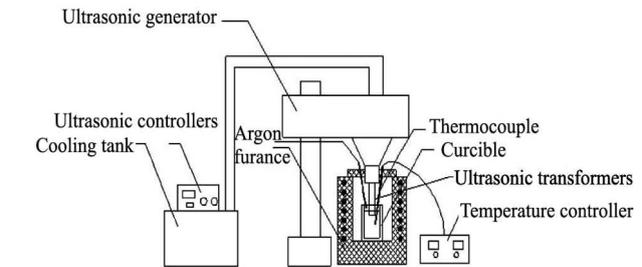
Fig. 1 Schematic of ultrasonic vibration device
