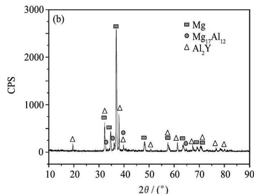
Fig. 2 XRD results of matrix of AZ91 (a) and  $\text{Al}_2\text{Y}/\text{AZ91}$  magnesium matrix composite (b)
